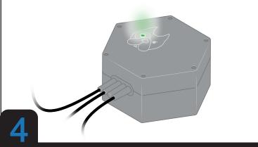
The MeterDog will continue to flash while establishing a secure connection. Activation is successful once the LED goes from solid green, then the LED turns off.
