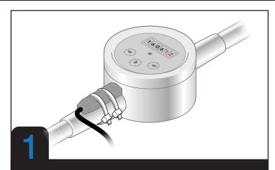
Step 1: Secure the MeterDog Sensor to the water meter register using the provided cable ties. Be sure the sensor tip is up against the meter register.
