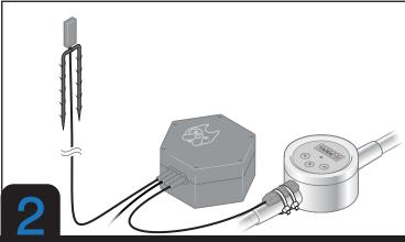
Position the antenna as high as possible to optimize cellular signal using the stake. Avoid installing the antenna tip on metal or on the ground
